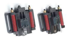
**Counterbore Tool Slide** - the counterbore slide module accessory bolts directly to the standard tool slide and can be installed immediately upon completion of the cut & external Be vel, to remove any internal inconsistencies prior to welding. The counterbore tool slide module is available in a range of travel lengths.
