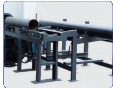
Pipe Conveyor System
