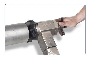
The Jaw system itself consists of 3 equilaterally positioned machined jaw segments, retained and locked on an inner, 'grooved' expansion shaft. These grooves keep the jaws held securely in position, unlike other systems that use a metal or rubber bands for jaw retention.
