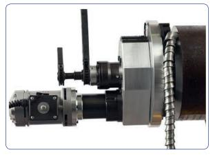
The Prep 20 has unrivalled power and stability, utlising a ratchet system for both jaw locking, and bevel feed.
