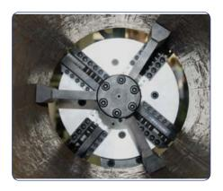
Innovative Wide locking jaws offer 6 point locking from 3 jaws giving superior clamping force for chatter free end preps.
