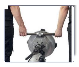
To enable ease of set up, the machine is equipped with a double-sided yoke with removable extensions so the machine can be easily installed, and removed from the pipe.
