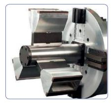
Self-centering 100mm (4") one piece locking shaft with build in jaws, eleminates the issue of broken or loosening retaining springs and o-rings.
