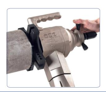
the Jaw system itself consists of 3 equilaterally positioned machined jaw segments, retained and locked on an inner, 'grooved' expansion shaft. these grooves keep the jaws held securely in position, unlike other systems that use a metal or rubber bands for jaw retention.
