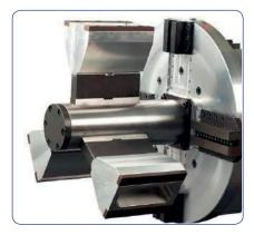
Self-centering 150mm (5.9") one piece locking shaft with build in jaws, eleminates the issue of broken or loosening retaining springs and o-rings.
