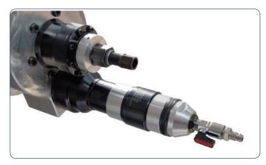
The PREP 20 can also be supplied as an electric version, with a 3200 watt heavy duty, in-line or right angle motor drive. Or a heavy duty 3.5 Hp Pneumatic motor
