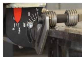
Continuous angle adjustment from 0 to 60 degrees.
